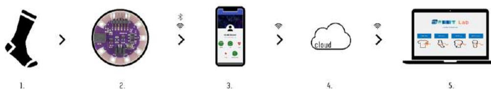
Figure 1. System Architecture: (1) SWEET Sock—Textile Unit; (2) SWEET Sock—Control Unit; (3) SWEET App; (4) Web Server; (5) SWEET Lab.
