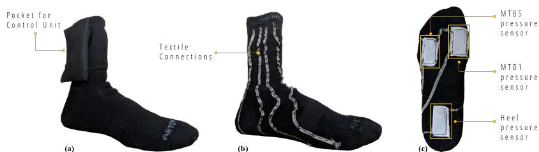
Figure 2. SWEET Sock sensing unit: (a) external view; (b) internal view of textile connections; (c) textile pressure sensors.
