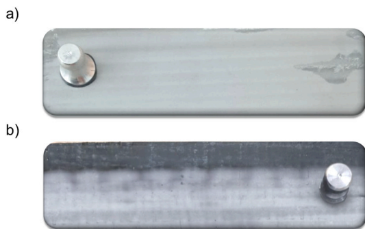
Fig. 5. Positioning of aluminum dolly for adhesion test on a) unreinforced substrate b) reinforced substrate.
