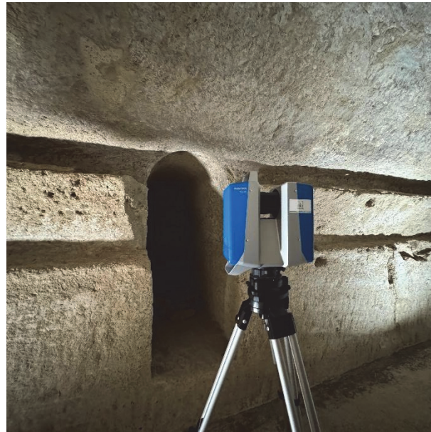
Figure 6. Acquisition phases with the Z+F Imager 5016A laser scanner.
