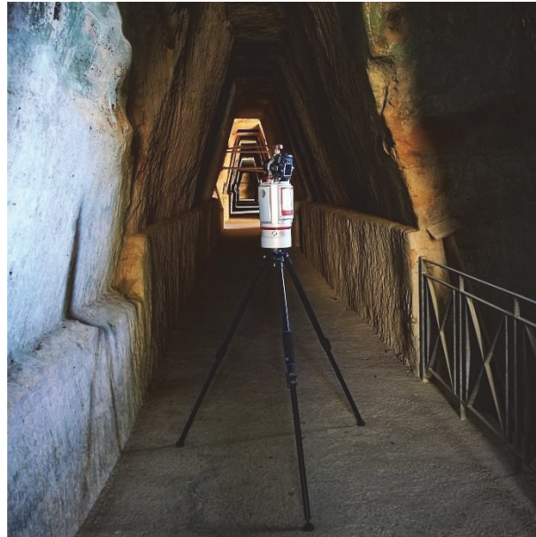
Figure 5. Acquisition phases using the Riegl VZ400i TOF scanner of the Antro della Sibilla .
