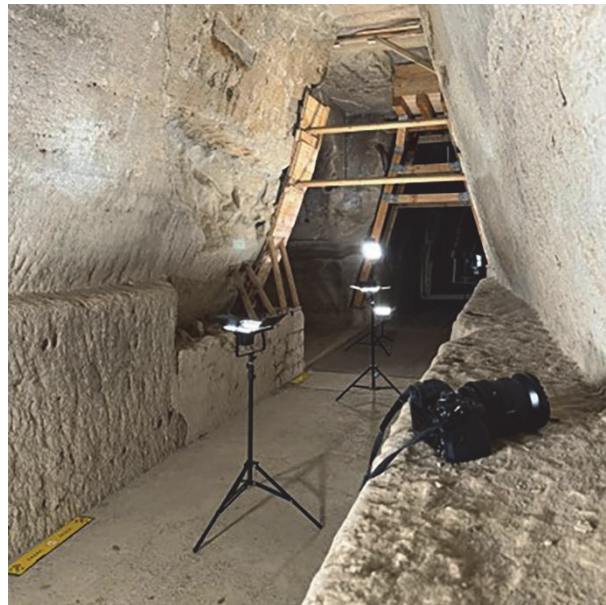
Figure 8. Photogrammetric acquisition phases with a Sony ILCE-7M4 camera.
