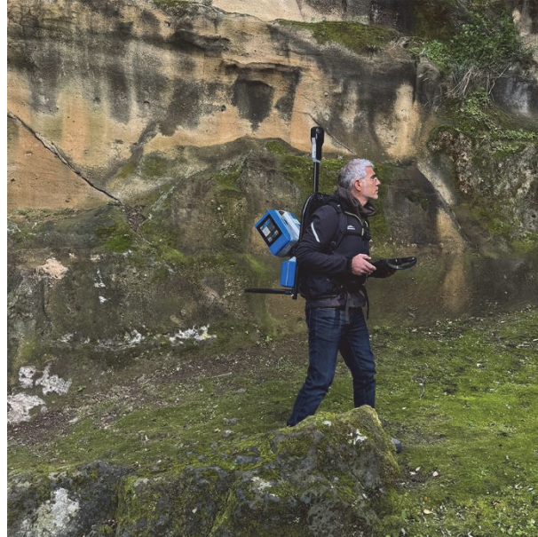
Figure 7. Acquisition phases with the ZF Imager 5016A laser scanner in dynamic mode.
