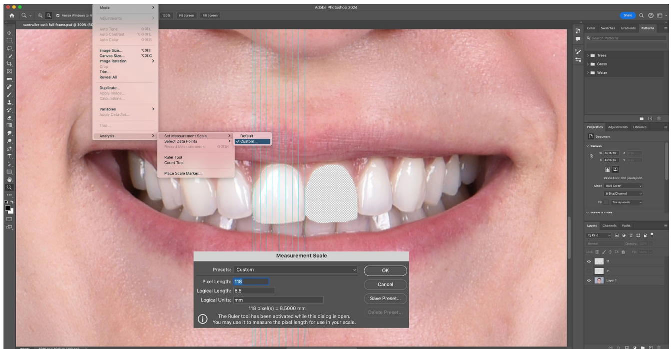
FIGURE 2 | Length calibration in photo editing software (Photoshop CC, Version 25.12.0).
