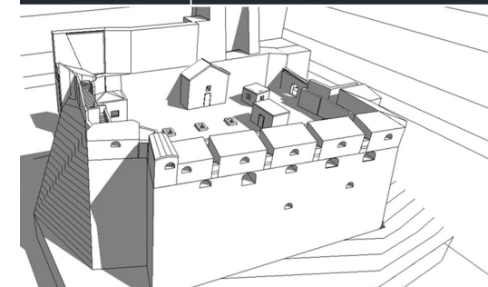
Fig. 10 - From top: definition of the levels preparatory to the scan-to-BIM procedures; a portion of wall and steps with complex geometries; some elements modeled with local families; H-BIM of Piazza d'Armi and fortifications
