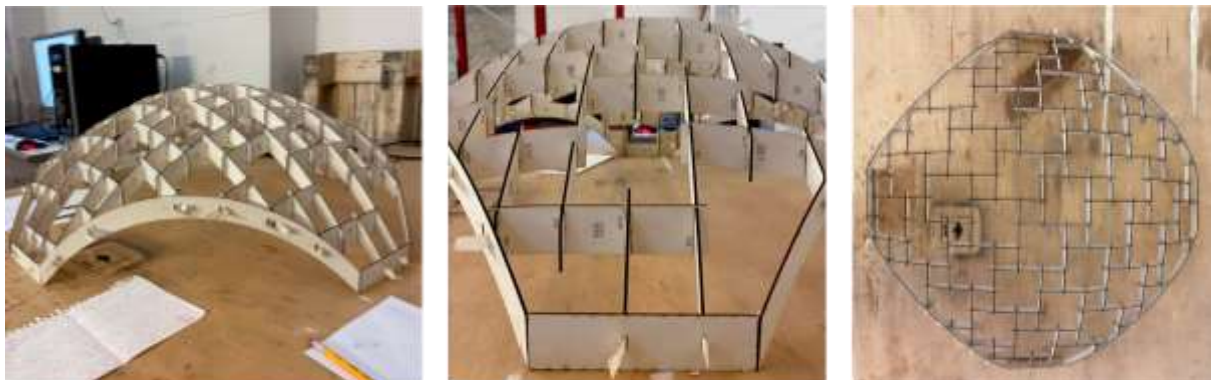
Figure 18: Assembly of the model completed with the addition of edge beams.
