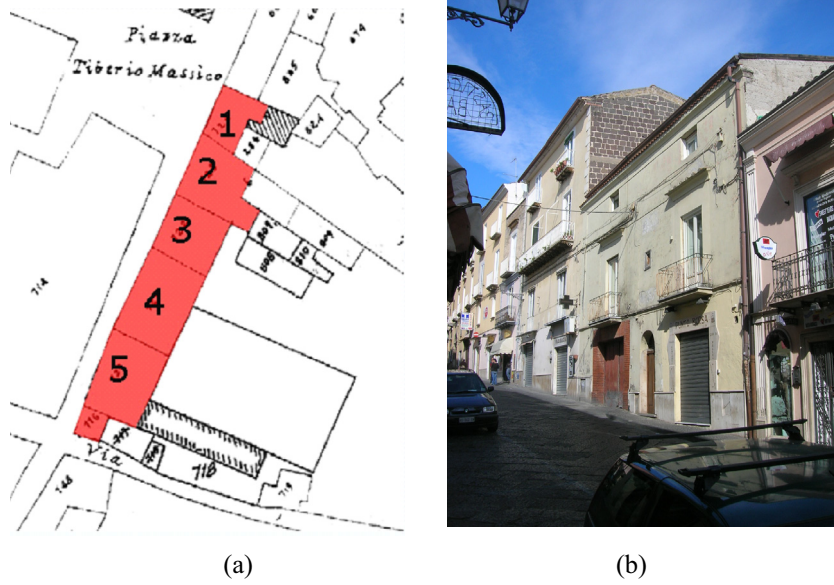
Fig. 21. The aggregate investigated in Sessa Aurunca: plan layout (a) and 3D view (b).
