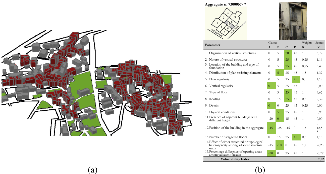
Fig. 40. Seismic vulnerability assessment of the historical centre of Poggio Picenze: the examined aggregates (a) and a typical form filled for a given aggregate structural unit (b).
