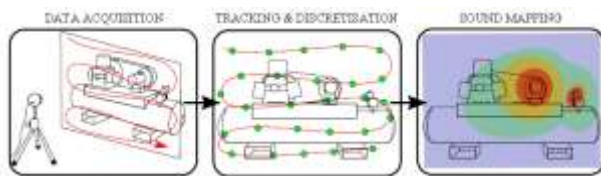
Fig. 6: Basic steps of the Scan & Paint measurement method
