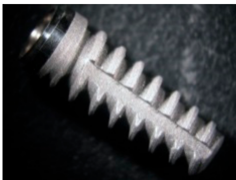
Figure 7. A picture of the dental implant covered by TiO 2 nanotubes [37].
