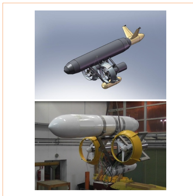
FIGURE 3 GEM prototype for towing tank tests. Scale 1:8
