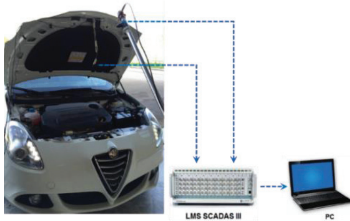
Fig. 1. Experimental layout – location of the microphones.
