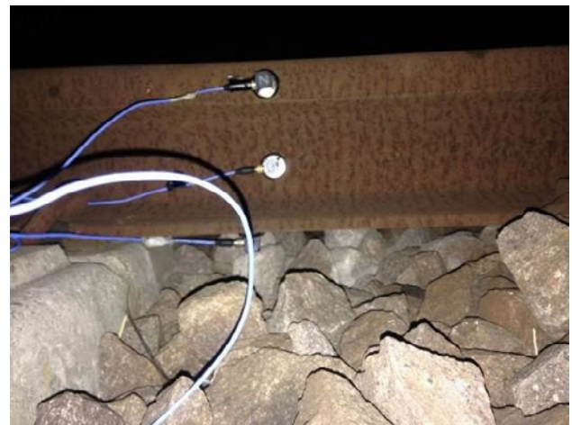
Figure 8 : Accelerometers positioned on the rail
