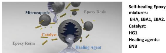
Fig. 2 Different compositions of self-healing systems [2]
