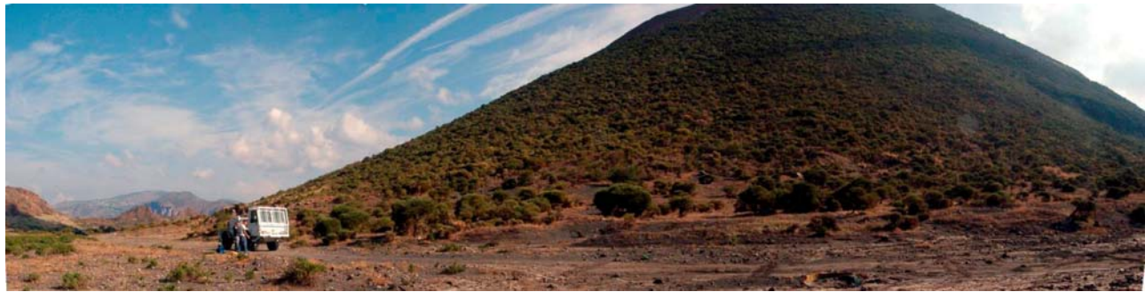
Figure 2. Photograph of the southeastern sector of La Fossa Caldera showing the Minivib during the acquisition of seismic profile FV2. Rough logistical conditions characterize the site; the soil is made up by dry and loose variable size sediments reworked from outcropping pyroclastic flows, fall, and lava beds. Visible on the right is La Fossa Volcano and, in the background at left, the northern boundary of La Fossa Caldera with Lentia Complex and Vulcanello (LC and LV in Figure 1).
