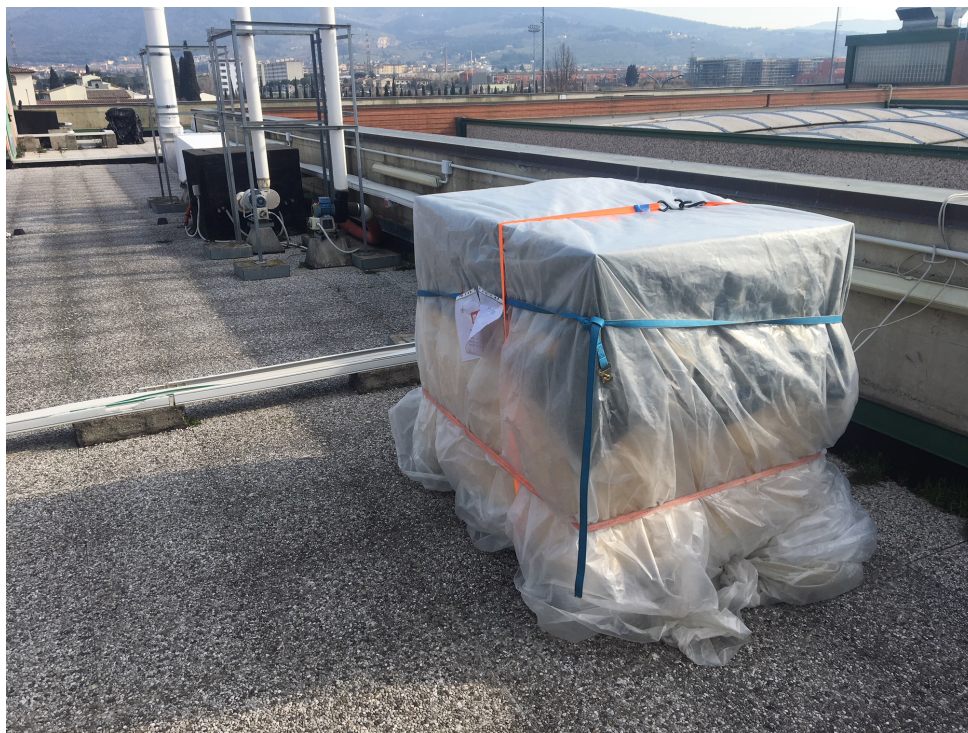
Figure 13. Installation of the MIMA hodoscope on the roof of the INFN building in Sesto Fiorentino (Firenze, Italy) for a measurement of the reference free sky vertical flux.
