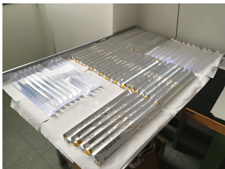
Figure 1. Left: the total set of scintillator bars with triangular section used for the MIMA tracking planes. Right: one module composed of X and Y planes under test.
