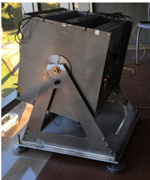
Figure 2. Left: the MIMA tracker under test after assembling three complete modules inside the mechanics. Right: the final MIMA telescope, provided of an altazimutal mounting, used for on-field measurements.
