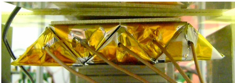
Figure 9. The five scintillator bars with triangular section used for the study of the spatial resolution achievable with the MIMA tracking planes.
