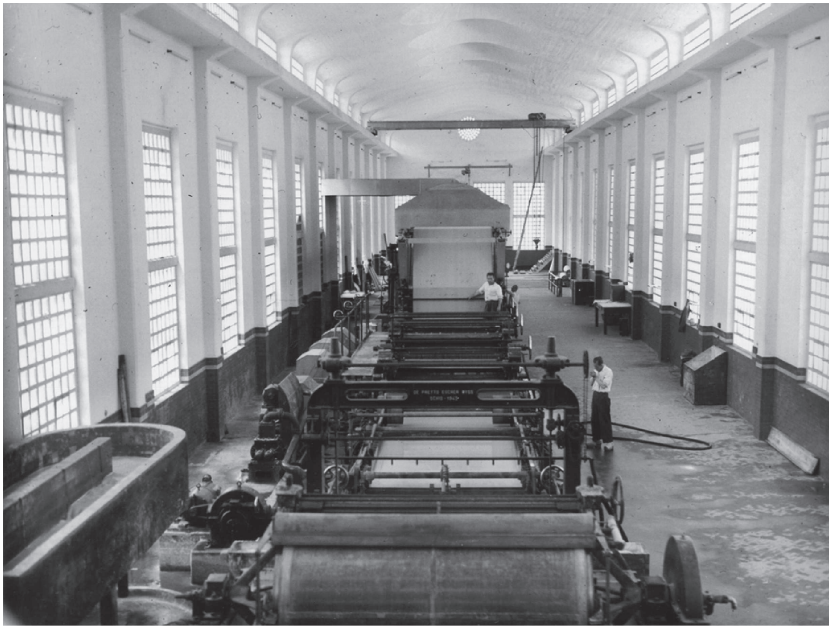
Fig. 16. Continuous machine. Atina's Paper mill. Taken from the Municipal Library of Atina
