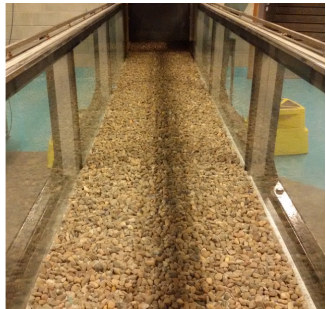
Figure 2. Installed gravels on the channel bed
