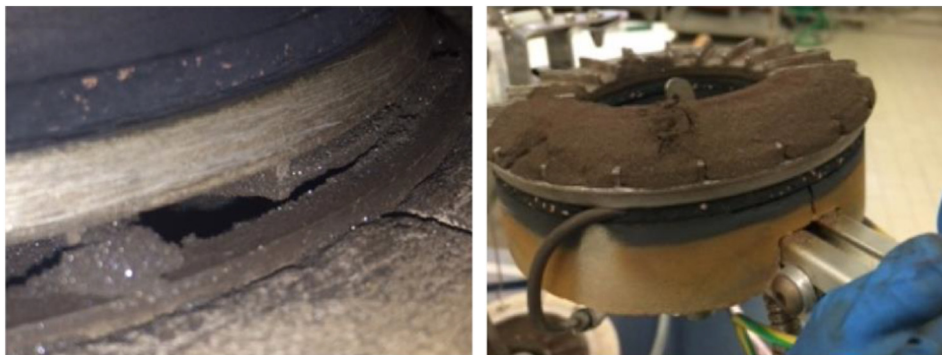
Fig. 12. Images of the cell during a test at a value of 1900 Pa of applied normal stress. On the left the lid lifted during the test. On the right the caked material in the lid vanes after the cell cooling.
