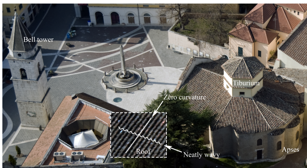
Figure 7. An aerial photograph allowing the addition of information lacking from the point cloud, such as the roof shape.
