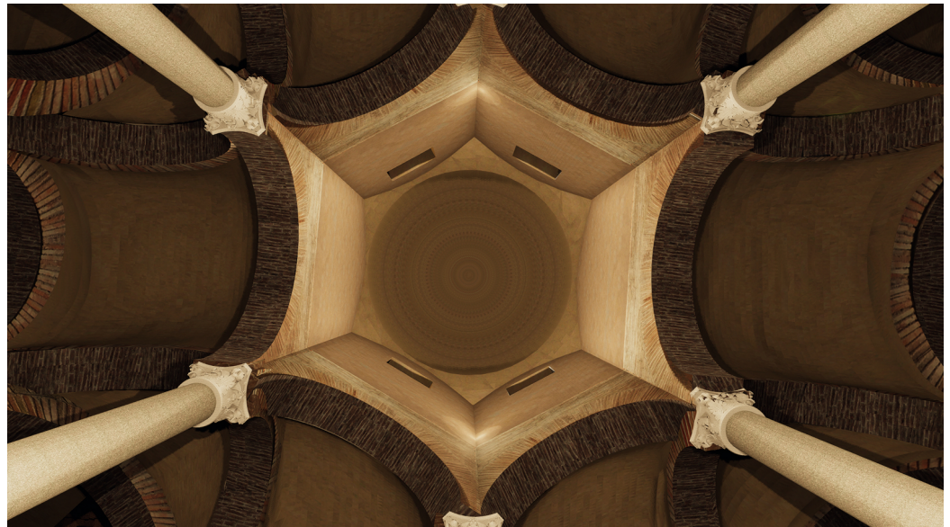
Figure 14. A rendered view of the tiburium and its ellipsoidal dome, taken from below.
