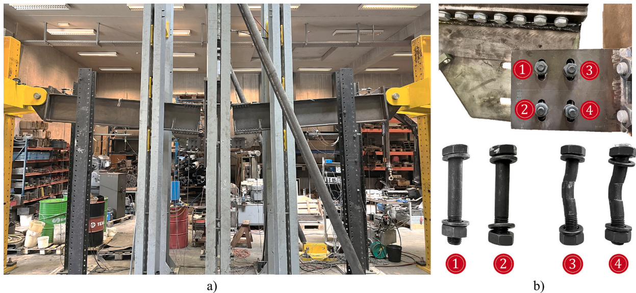
Fig. 10. – Test 2 – Experimental response: a) Deformed specimen after test; b) Friction damper and damage of damper bolts after test.
