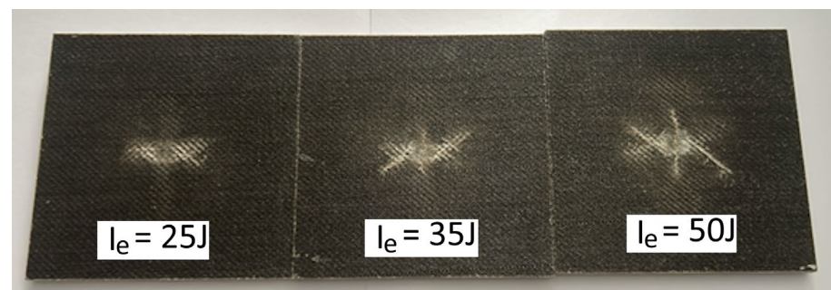
Figure 9. Pictures of the indentation damage that occurred on the IP 12 specimens, impacted with three different levels of impact energy I_e .
