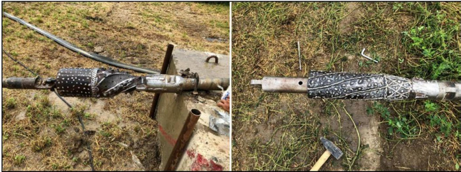
Fig. 26 Adopted reamer for HD (left) and IPS (right)
