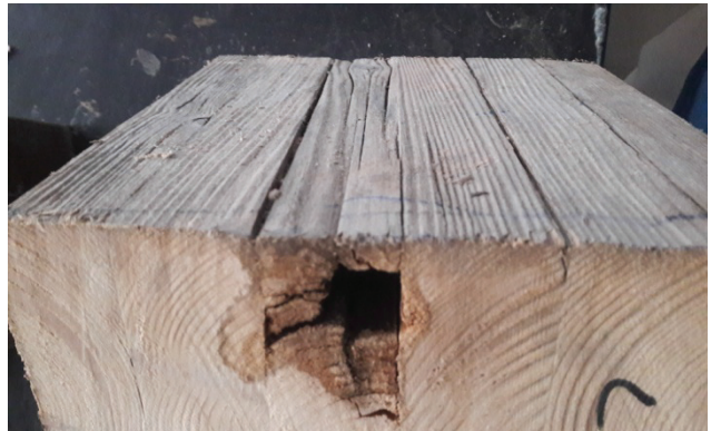
Fig. 6 – Degradation in a cross section
